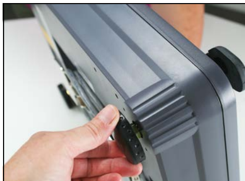
Figure 2-4. Adjust the Scale Base Feet
