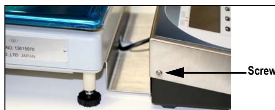
Figure 2-20. Indicator Attached to the Scale Base (DIGI S-YC Scale Base Shown)
